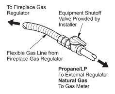
Figure 22 - Attaching Flexible Gas Lines
